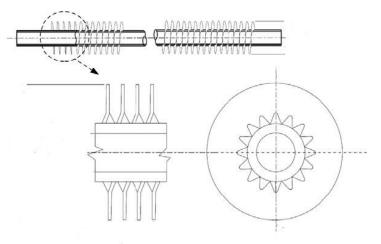
Crimped fin tube actual tubes supplied to the customer
