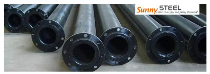
Bi Metal Clad flanged pipe is cast with mold vanishing vacuum suction casting cladding process.
