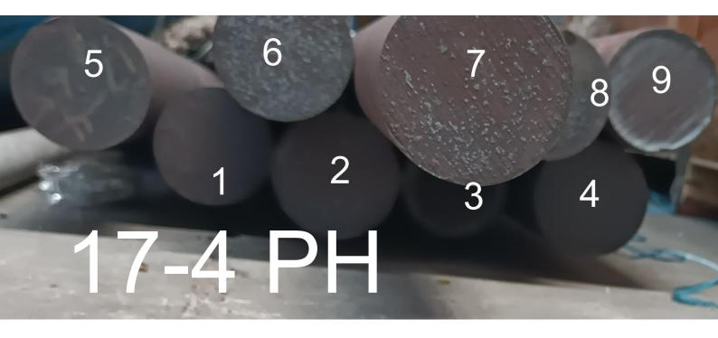
17-4PH is a precipitation hardened (PH) martensitic stainless steel consisted of copper and niobium/tantalum. This grade features high strength, hardness and corrosion resistance. Its mechanical properties can be optimized by heat treatment with the compression strength achieving up to 1100-1300mpa (160-190ksi). Due to low carbon content, it features better workability, corrosion resistance and weldability than Martensitic Stainless Steels such as Cr13 and 9Cr18 and 1Cr17Ni2.
